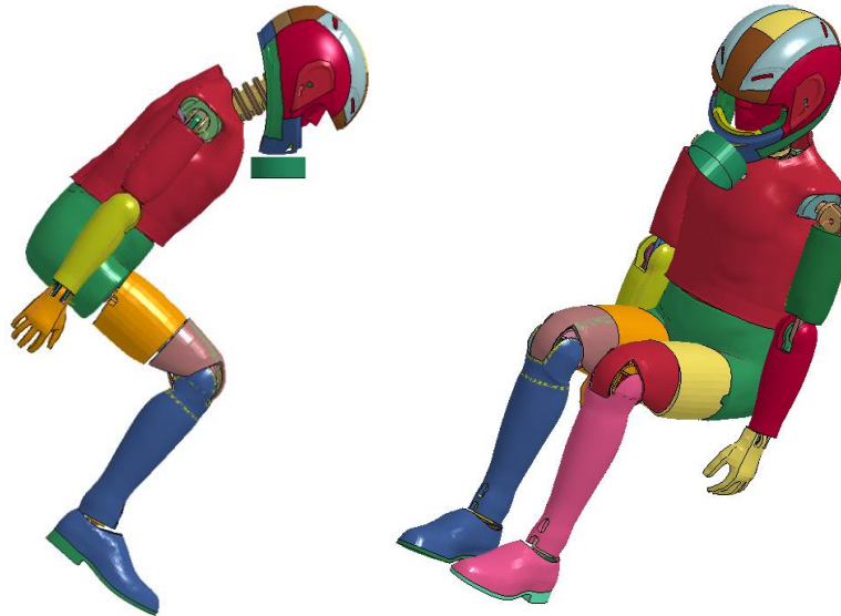
Fig.7: Helmeted Dummy model impacting a flat anvil.
