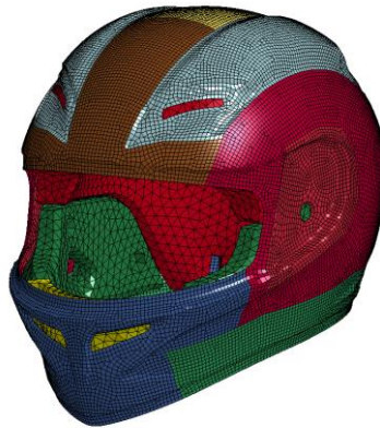
Fig.4: Helmet FE Model
