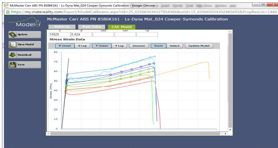
Fig.1: Material model calibration of ABS tensile data to MAT_024 CP using Matereality CAEModeler
