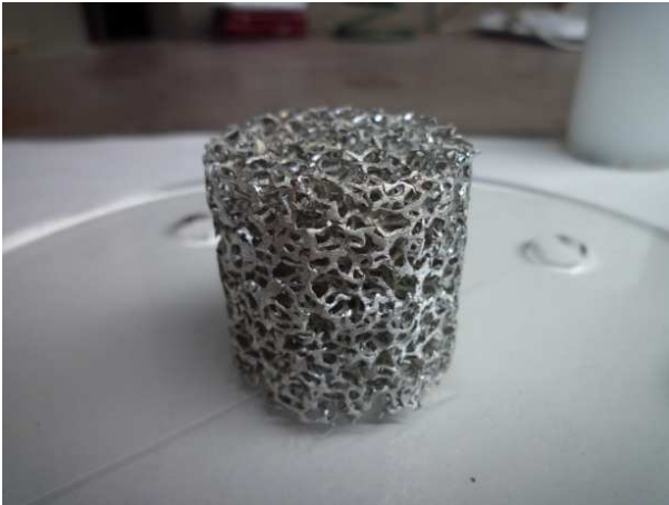
Figure 2: Cylindrical foam sample (d = 35 mm; h = 35 mm)
