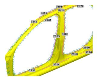
Figure 10 – Side panel frame and side impact related spot weld lines
