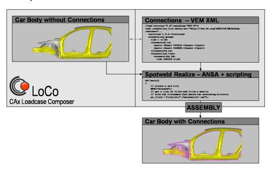
Figure 3 – Model assembly process with automated connection realization
