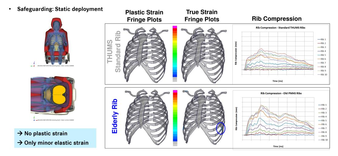
System performance: **Dynamic results**  $\rightarrow$  Old rib material **IIHS Barrier Test** 50 kph
