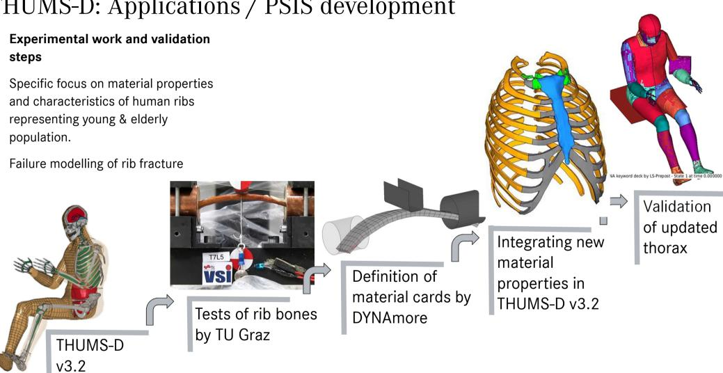
• Experimental work (TU Graz) (2nd test phase: female 32 years old & female 58-65 years old - 28 rib specimen)
