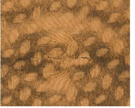
Plate consisting of 12 layer carbon fabric and rubber layer in the middle: damage after impact loading
