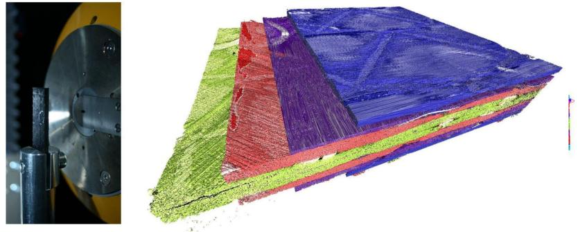
using fibre orientation analysis of VG all 8 layers of the UD-fabric can be extracted: 0/90/+45/-45/-45/+45/90/0° fibre orientation.
