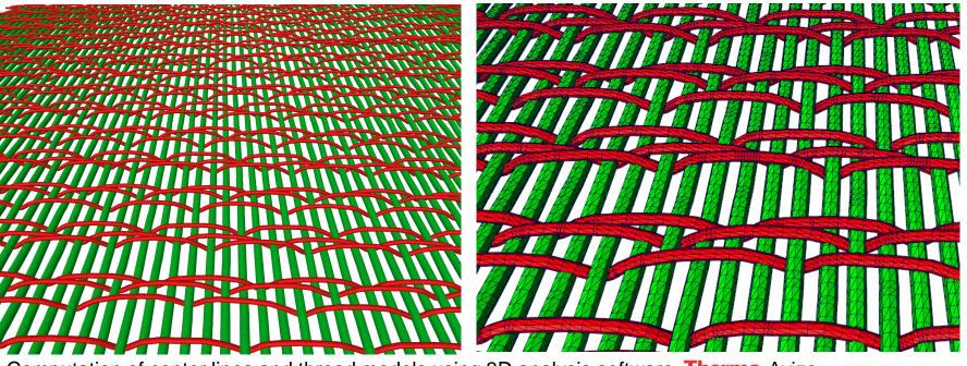
Computation of center lines and thread models using 3D analysis software Thermo Avizo
