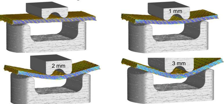
Analysis of four  $\mu\text{CT-Scans:}$  unloaded and at 1-3mm deflection of the sample
