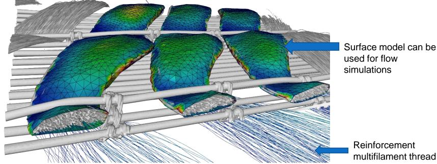
Computation of center lines and surfaces of multifilament ORW-threads and FE-modeling using Avizo ARENA2036 DigitPro
