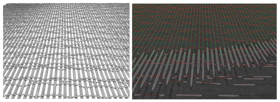
Computation of center lines and thread models using 3D analysis software Thermo Avizo ARENA2036 DigitPro
