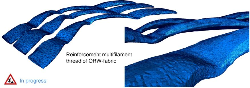
FE-model of mulitfilament threads meshed by tetrahedra volume elements (coarse & fine) using Avizo ARENA2036 DigitPro
