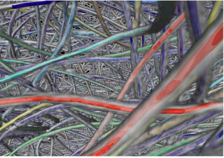
fiber segmentation and determination of fiber length by 3D-analyzing software Thermo Scientific Avizo
