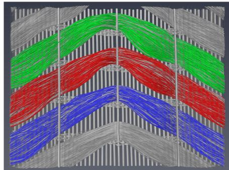
Computation of center lines and thread models using 3D analysis software Thermo Avizo
