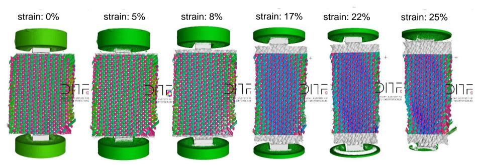
CT-Analysis of an Open Reed Woven (ORW)-fabric out of glasfiber rovings loaded at different tensile stages, color show fibre orientation angle
