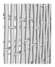
Fabric out of monofilaments: CT-scan 16,5 mm x 20,9 mm, resolution 7,5  $\mu m$
