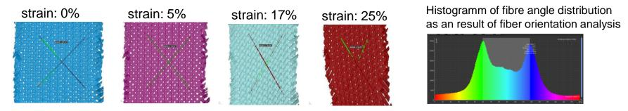
shear angle and lateral contraction over strain
