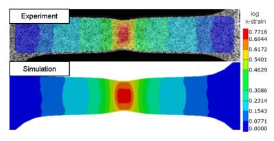
Deformation field of tensile test
