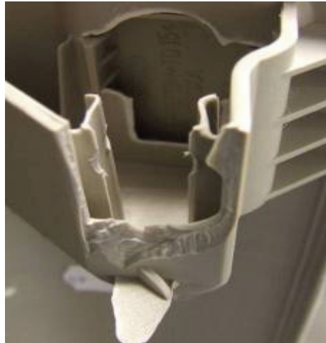
Figure 3 Common failure mode – local trim break
