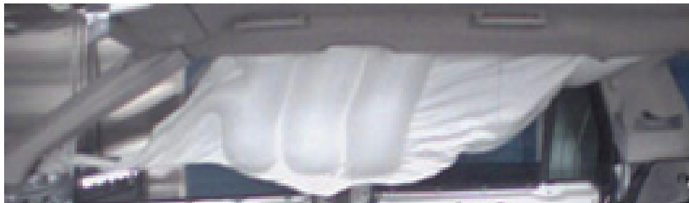
Figure 1 Common failure mode – curtain airbag hang-up
