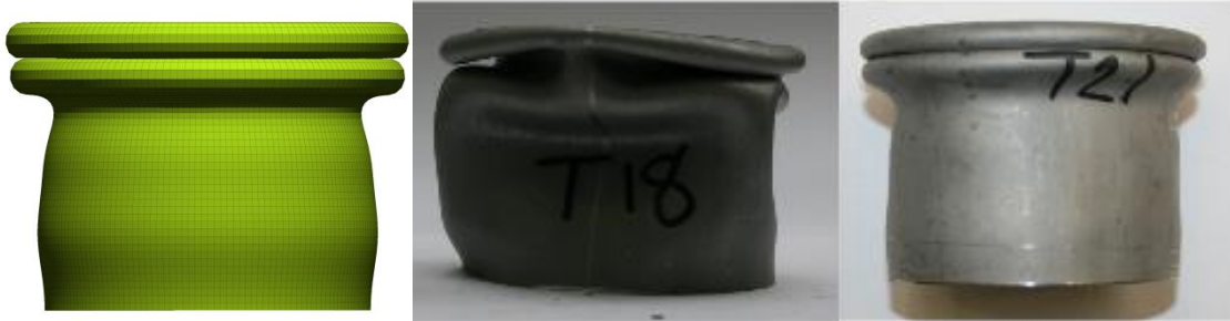
Fig. 2: Final deformation of 2½"Sch5 pipes in FEA (Left), typical deformation (Mid) and from Test 21 (Right)
