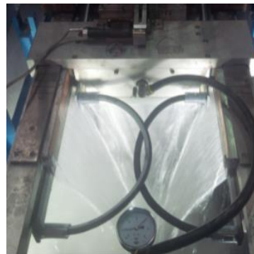
Fig.2: Water flow in a CC mould
