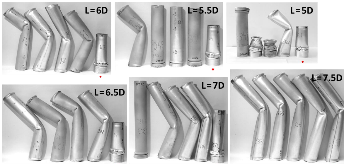
Fig.11: Five parallel tests that show the deformation mode for different length 5D < L < 7.5D .
