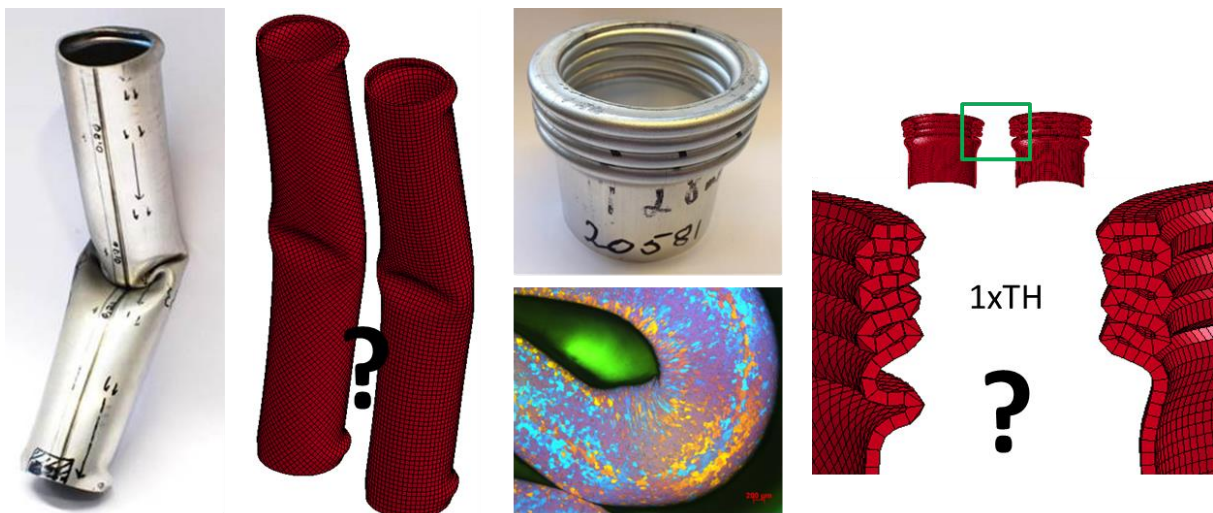
Fig. 14: A numerical model based on cubic shaped solid elements does not predict all relevant details.
