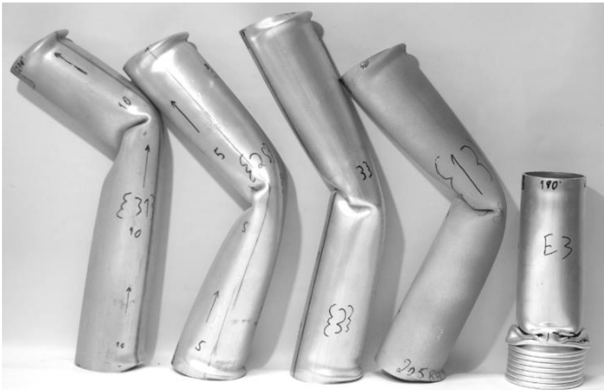
Fig.8: Results with the sensitive geometry defined with length, diameter and thickness L = 6D = 180T .
