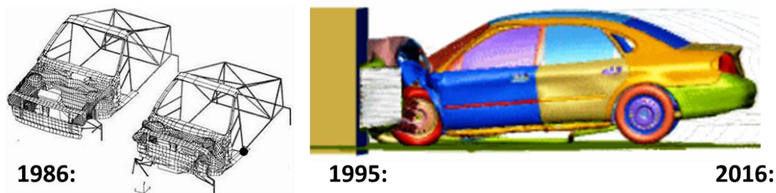
Fig.1: Increased computational power has resulted in FEM models with more elements and details.
