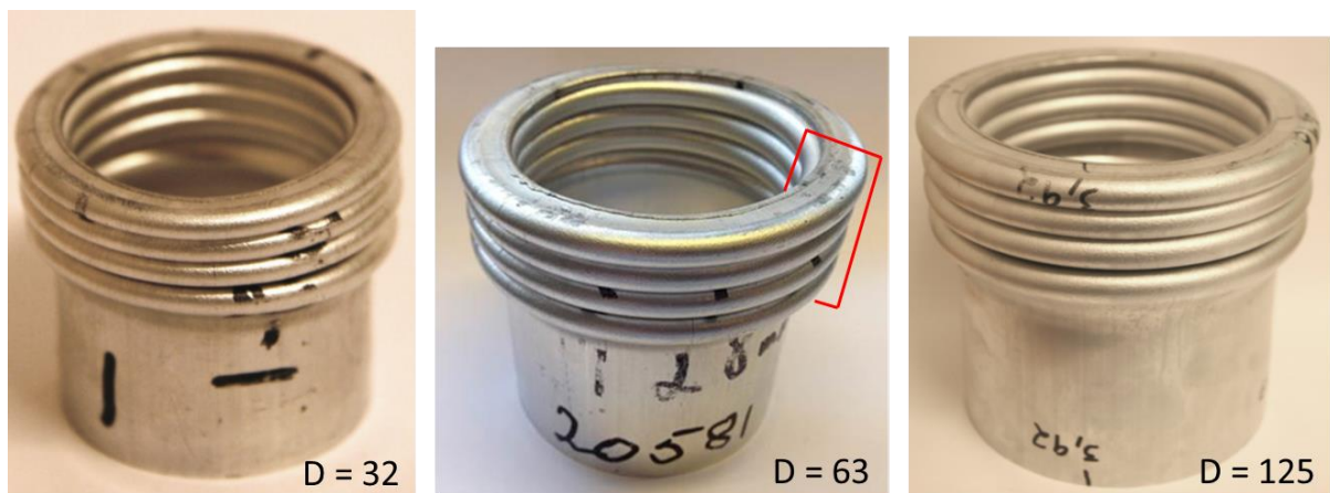
Fig.6: Specimens with L = 2D = 60T shows four concertina rings when compressed into half-length.
