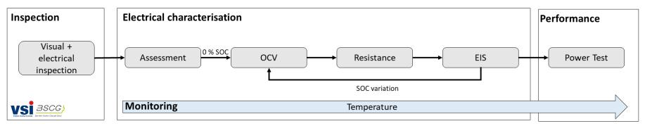
• Multi-step test protocol → a programmable cycling station is used
